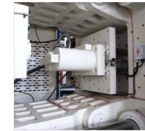
双顶针缸结构 Double ejector cylinder structure
