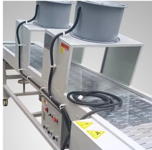
耐高温输送带 High temperature resistant conveyor belt
