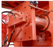
一体式双顶针缸 One-piece double ejector cylinder
